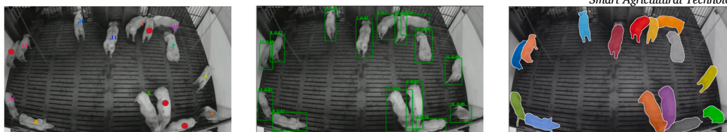
Fig. 4. Visual comparison of detection performance between idTracker (left), PromptTrack (center), and Track-Anything (right). (left) idTracker snapshot showing several undetected animals (marked with red points). (center and right) Track-Anything and PromptTrack snapshots showing all animals detected.
